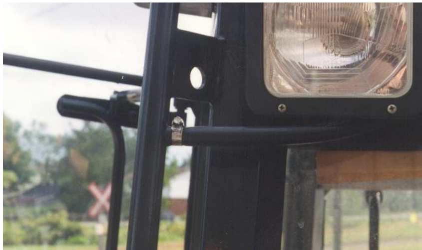
Drain tube locations and set-ups.
